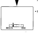
"DETECTING TAPE POSITION" is only displayed when a cassette is first inserted. It takes several seconds for correct tape position to appear.
